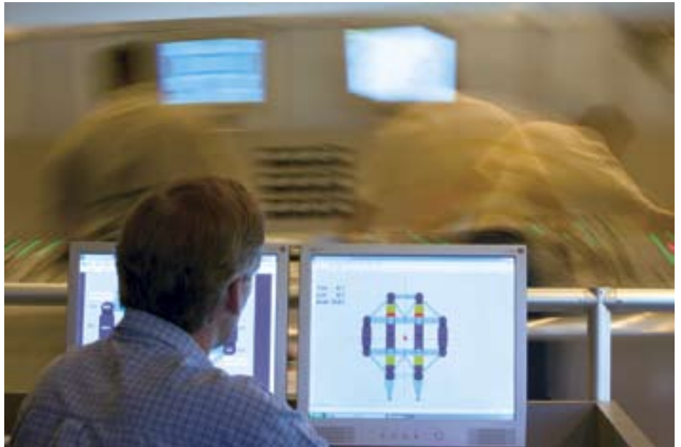
Top photograph, a mock ballast-control room—one of only two in the world—mounted hydraulically, simulates the action of wind and waves on an offshore rig. Center and bottom, roustabout trainees on the Mr. Charlie.
